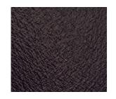
A revolution in leak detection, this is a geomembrane with a fully integrated electrically <u>conductive</u> bottom surface. This allows quality teams to conduct a spark test immediately following installation and a dipole survey after the liner is covered.
