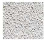
Our White Reflective reflects solar radiation to keep the liner cooler, resulting in fewer wrinkles, while facilitating damage detection and eases installation.
